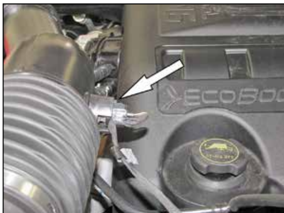
2. Disconnect the Inlet air temperature sensor electrical connection.
