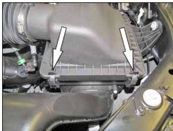
4. Release the two clips securing the upper air filter housing.
